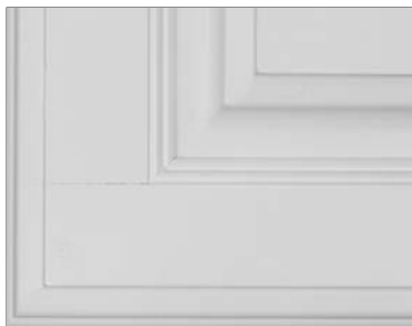
Example of front joint separation
