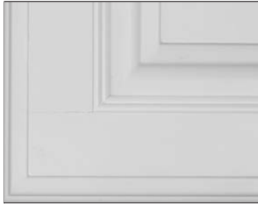
Example of front joint separation
